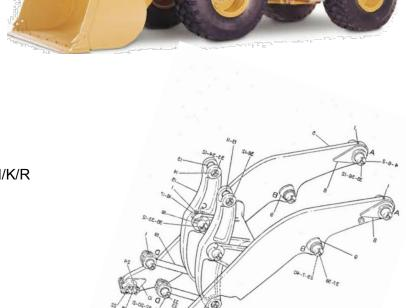
Our implement or bucket control parts are manufactured using the most modern systems of design, production, heat treatment and quality control to give lasting results in the field. Providing the correct through hardness of those surfaces subject to wear, is key to providing abrasion resistance and shock load impact. CGR. Manufacturers of Caterpillar parts since 1962.
